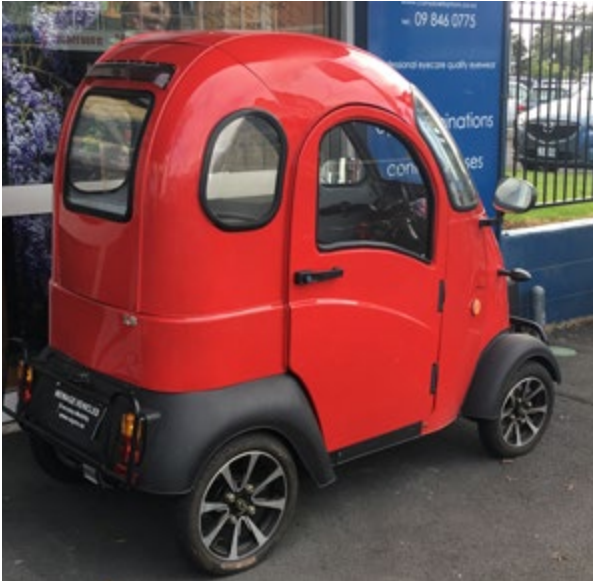
Figure 3-16: Newage B4: 1000-watt motor, range 40 km to 160 km, top speed 30 km/h (Source: Newage Vehicles)
