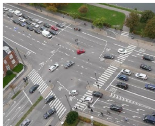
Figure 6-42: Possible road marking to create 'box turns' for MS lane users at an intersection
