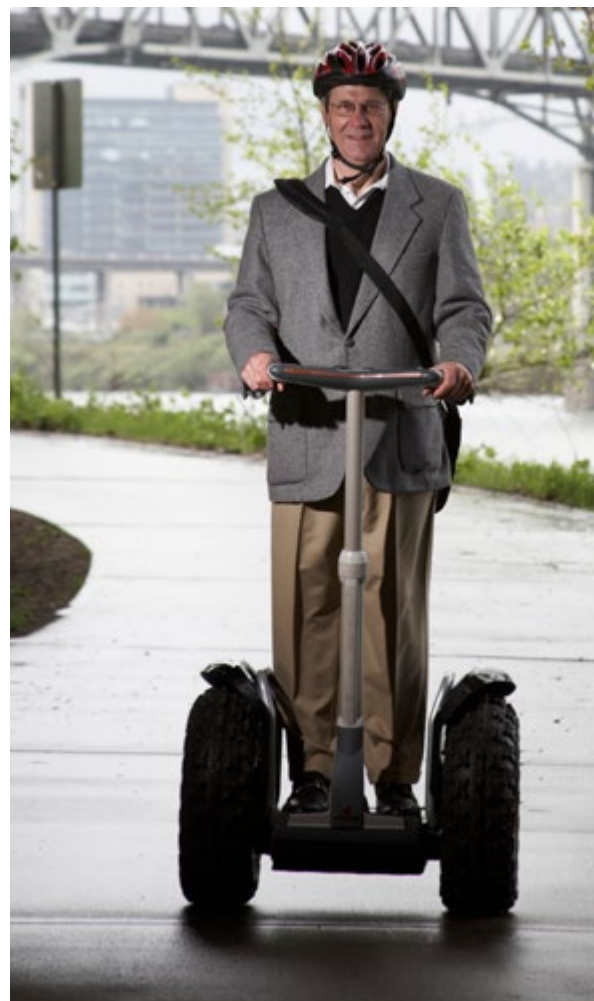
Figure 3-6: Segway PT 2 x 750-watt motors, range 20 km, topspeed 20 km/h
