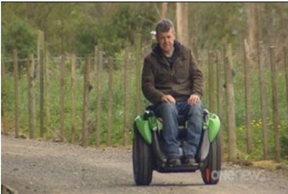
Figure 3-8: Ogo self-balancing wheelchair (Source: One News, TVNZ)
