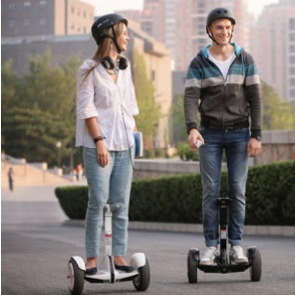
Figure 3-7 Segway Ninebot mini pro 2, 2 x 800-watt motors, range 30 km, top speed 18 km/h (Source: Segway)
