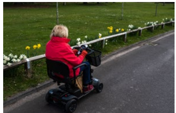
Figure 3-15: Standard mobility scooter: up to 1500-watt, range 30 km, top speed 16 km/h
