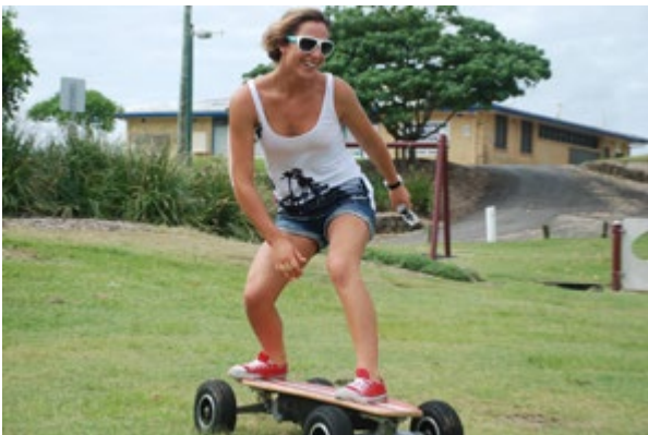
Figure 3-13: FiiK Street Surfer, range 30 km, top speed 37 km/h, regenerative antilock braking (Source: FiiK Skateboards)
