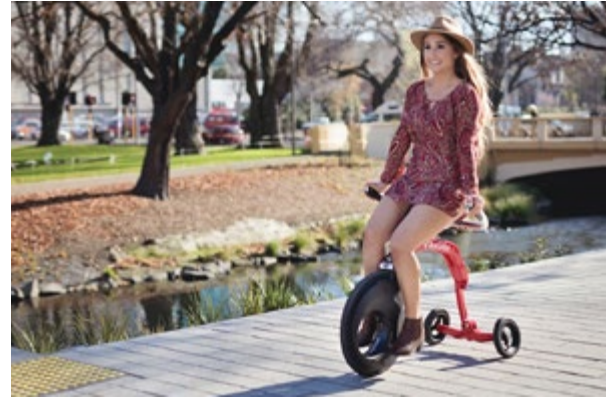
Figure 3-9: YikeBike model C: 200-watt motor, range 20 km, top speed 23 km/h (Source: YikeBike)
