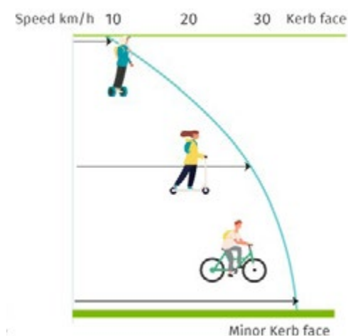
Figure 4-30: Sketch of proposed speed profile of Medium Speed Lane(MS)
