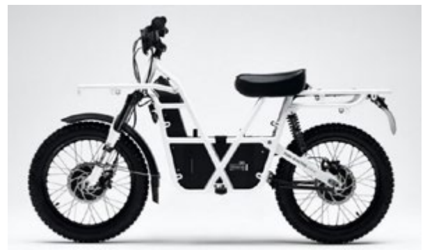
Figure 3-19: UBCO: 2000-watt, range 120 km, top speed 50 km/h (Source: UBCO Bikes NZ)
