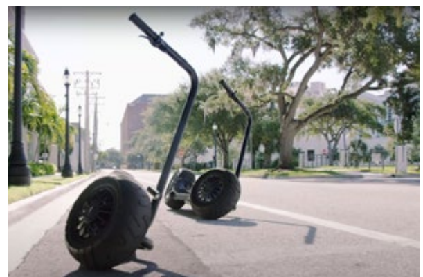
Figure 3-11: Stator 'self-balancing electric bike' 1000w motor, range 32 km, top speed of 40 km/h (Source: NantMobility)
