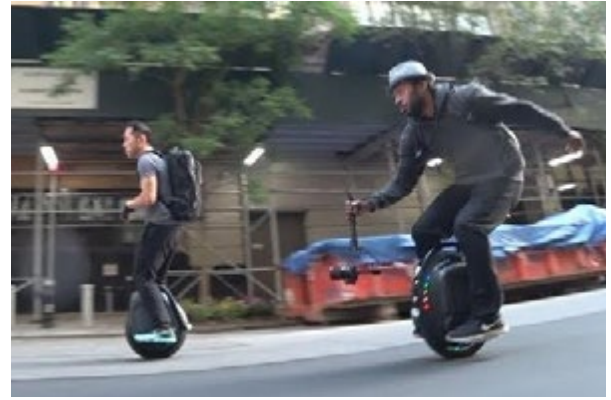
Figure 3-14: Ninebot One Z10: 1800-watt, range 90 km, top speed 45 km/h (Source: Citi Wheel)
