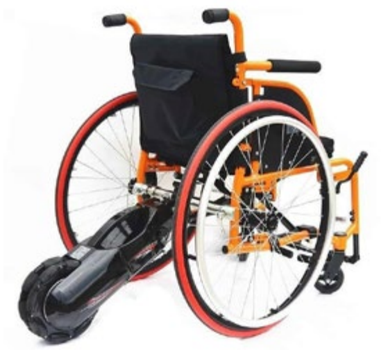
Figure 3-17: Electric Wheelchair Tractor: 250-watt motor, range 30 km, top speed 7 km/h (Source: EJOYQ)
