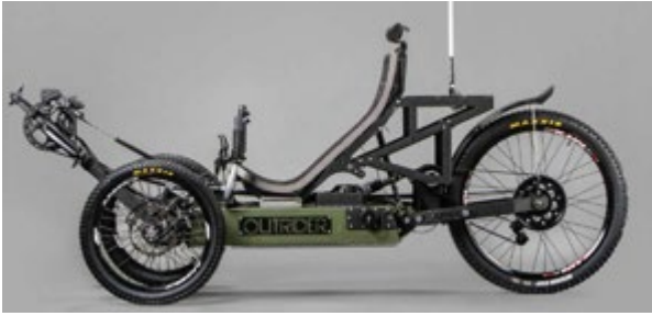
Figure 3-20: Outrider recumbent e-trike 4200-watt max, 750-watt continuous, range 320 km, top speed 56km/h. (Source: Outrider)
