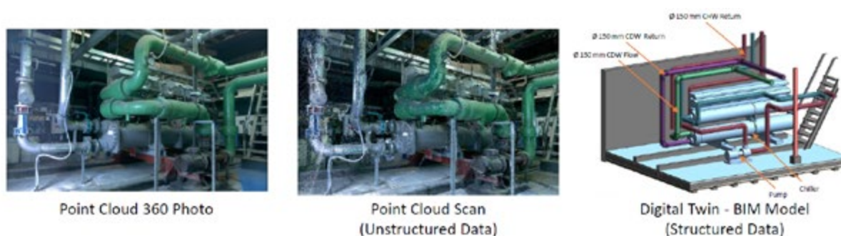
Fig 11: Example of a single location point cloud survey combined with a 360-degree image used to create a digital twin (Image courtesy of Nikhil Makan, Aurecon Christchurch office)
